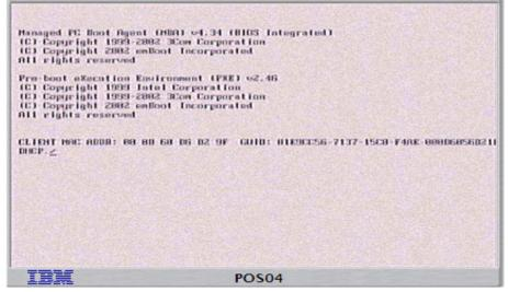
Figure 5-26 POS system booting up from the network
